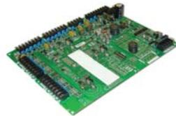
Uses MEP to MODBUS converter developed by SLS
